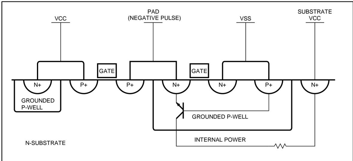
The P-well is held at ground, so the parasitic NPN transistor should never turn on. If, though, a negative pulse is applied to the pad, and hence to the emitter of the parasitic NPN transistor, the transistor would be put into its conducting mode. Once the pad is taken to  $-V_{be}$ , the parasitic bipolar transistor turns on, and pulls current from the substrate.
