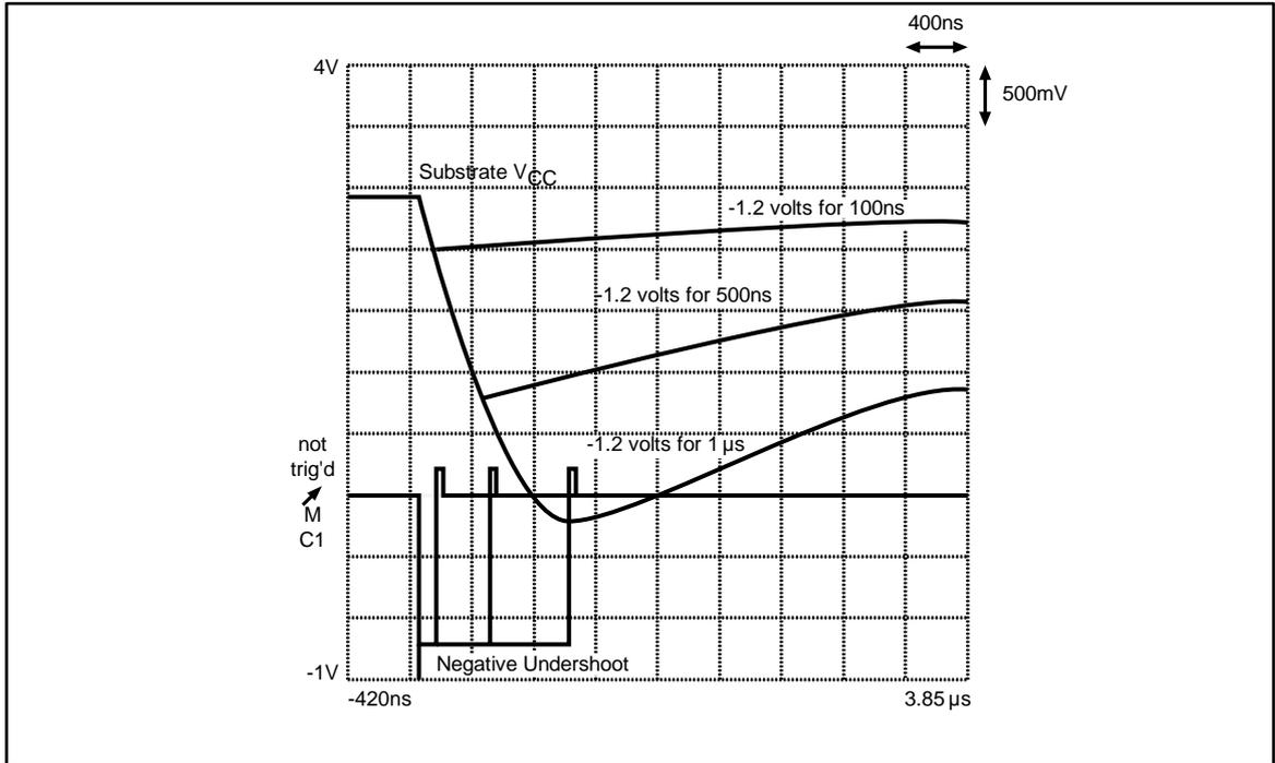
Figure 2: "Substrate  $V_{CC}$  versus negative undershoots" superimposes three pairs of curves: three negative undershoot pulses of 100, 500 and 1000 ns duration; and the corresponding effects that are felt by the  $V_{CC}$  substrate voltage.
