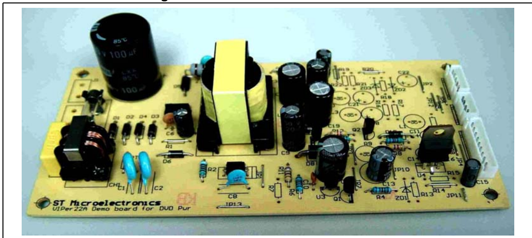
Figure 1. VIPer22A-E evaluation board
