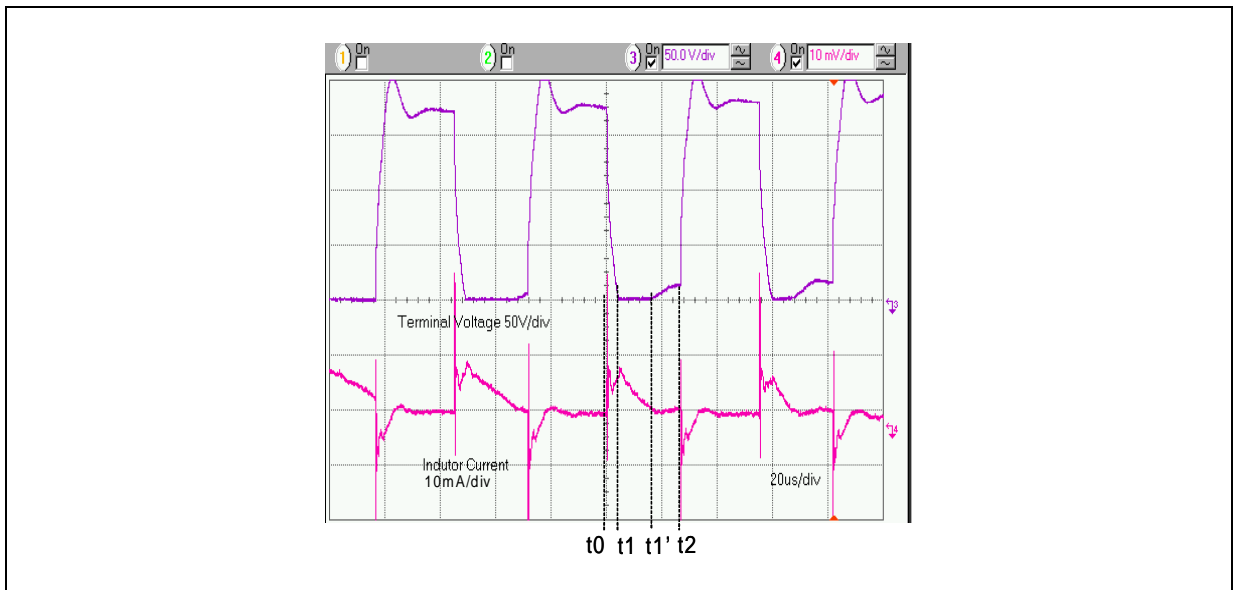
Figure 5. Waveform of floating phase terminal voltage and inductor current
