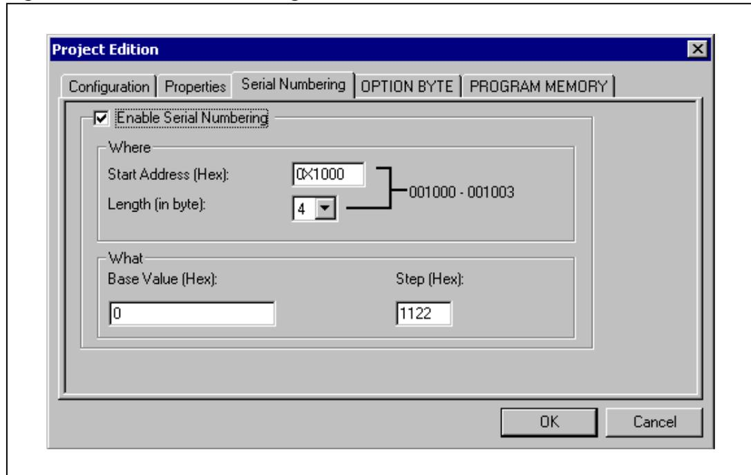
Each time a new chip is programmed, the current 'base value' is programmed at the 'start address' location, over 'length' bytes, and then the 'step' is added to the 'base value', forming the new 'base value' for the next programming cycle.
