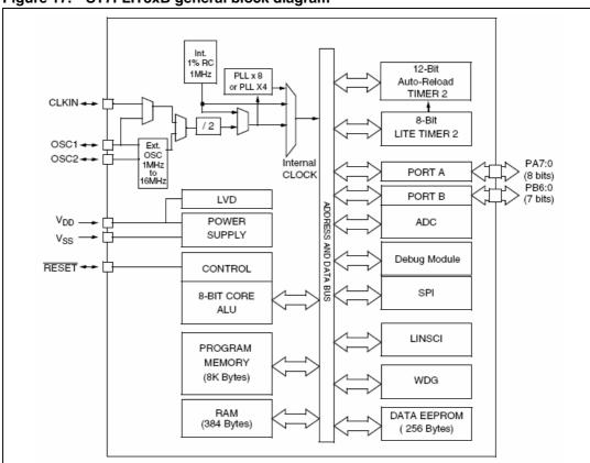
Figure 17. ST7FLIT3xB general block diagram
