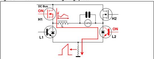
Figure 9. Inductor current during charge phase
