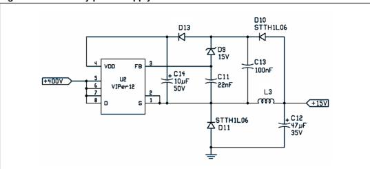
The VIPer12A-E is a low-cost smart power device with an integrated PWM controller that is suitable for such applications.
