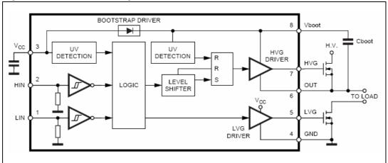
The L6385 is a high-voltage device, manufactured with BCD "OFF-LINE" technology. It has a driver structure that enables to drive independently referenced N-Channel Power MOSFETs or IGBTs. The upper (floating) section is enabled to work with voltage rail up to 600 V. The logic inputs are CMOS/TTL compatible for easy interfacing with controlling devices.
