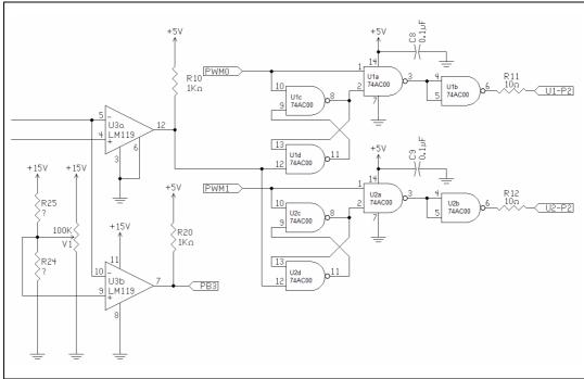
Figure 26. Current regulation circuit
