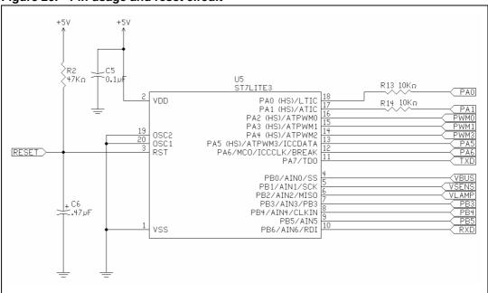
Pin 4: ADC channel 0 analog input, to measure the main DC bus voltage (VBUS). A
