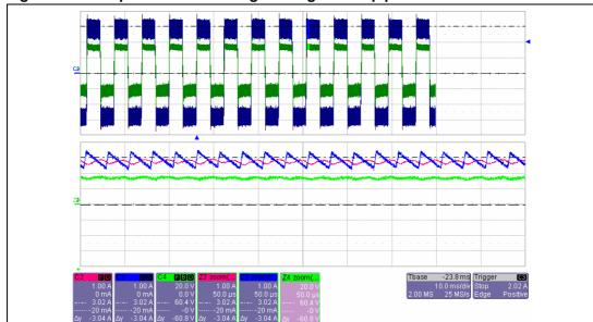
Figure 35. Lamp current and voltage during warm-up phase
