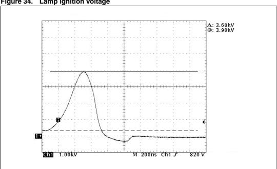
Figure 34. Lamp ignition voltage
