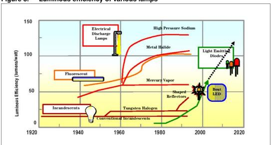
Figure 3. Luminous efficiency of various lamps
