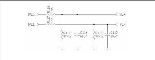
Figure 23. Lamp voltage measurement circuit
