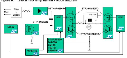
Figure 8. 250 W HID lamp ballast - block diagram
