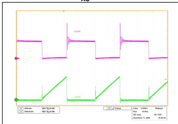
Figure 8. Drain current and voltage at full load 90 V AC
