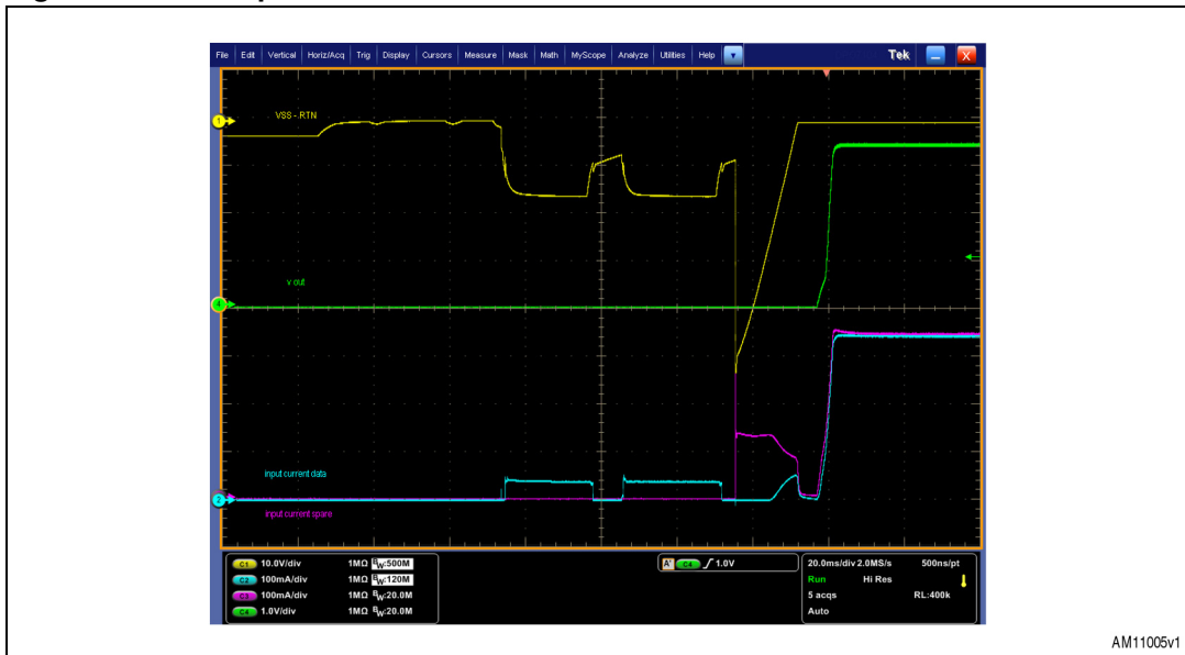
Figure 8. Startup with 10 A load
