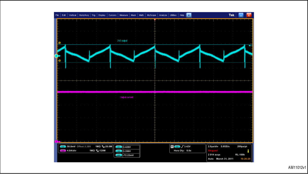
Figure 15. Output ripple measurement at 16 A with infinite persistence
