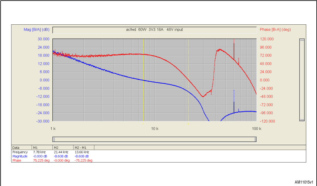
Figure 16. Control loop of the converter at 48 V input and 18 A output
