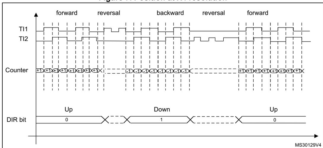
The timer's counter is incremented or decremented for each transition on the selected input TI1 or TI2.
