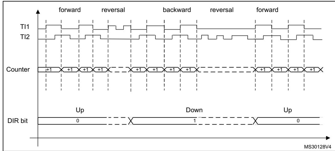
*Note:* In case of X2 resolution, the counter can also be incremented on the TI1 edge.
