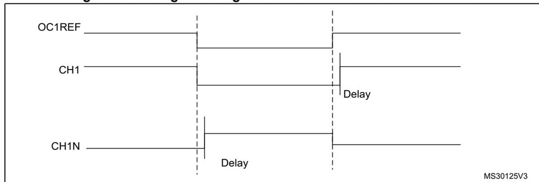
*Note:* The deadtime parameter is computed using the DTG[7:0] bits and the deadtime clock (Tdtg).
