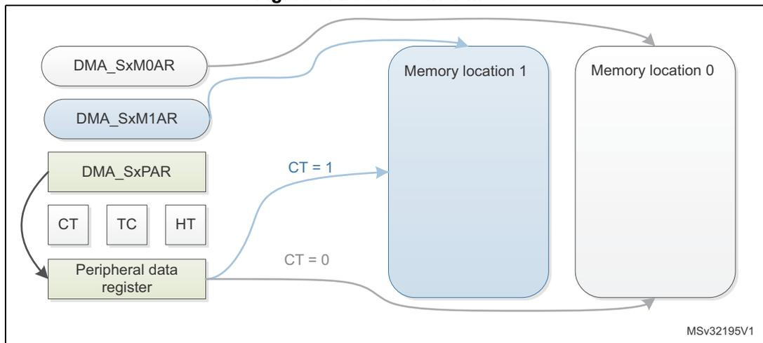
In Double-buffer mode, it is possible to update the base address for the AHB memory port on-the-fly (DMA\_SxM0AR or DMA\_SxM1AR) when the stream is enabled:
