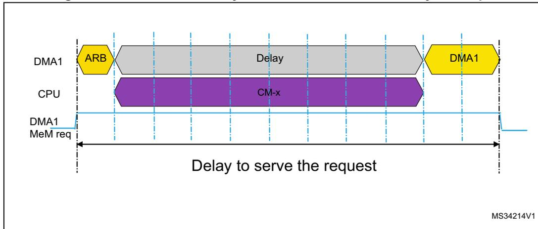
The above figure details the case of a DMA transfer delayed by a CPU multi-cycle transfer due to an interrupt entry. DMA memory port is triggered to perform a memory access. After arbitration, AHB bus is not granted to DMA1 memory port but to CPU. An additional delay is observed to serve the DMA request. It is 8 AHB cycles for a CPU transfer issued by interrupt.
