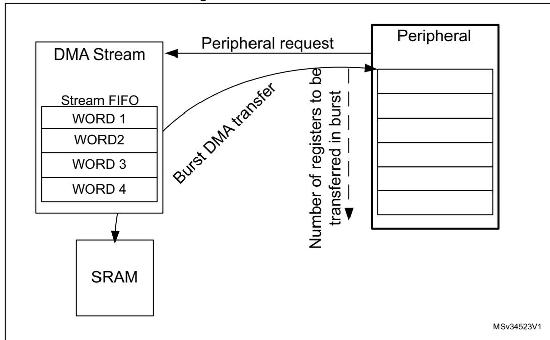
In response to a burst request from peripheral DMA reads/writes the number of data units (data unit can be a word, a half-word, or a byte) programmed by the burst size (4x, 8x or 16x data unit). The burst size on the DMA peripheral port must be set according to the peripheral needs/capabilities.
