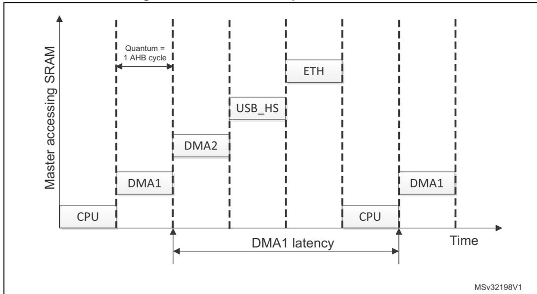
The latency associated to DMA1 to win the bus matrix again and access SRAM1 (for example) is equal to the execution time of all pending requests coming from the other masters.
