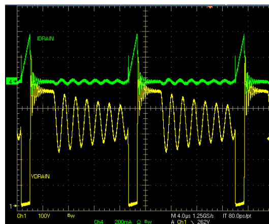
Figure 11. Drain current and voltage at 230 V AC , max load
