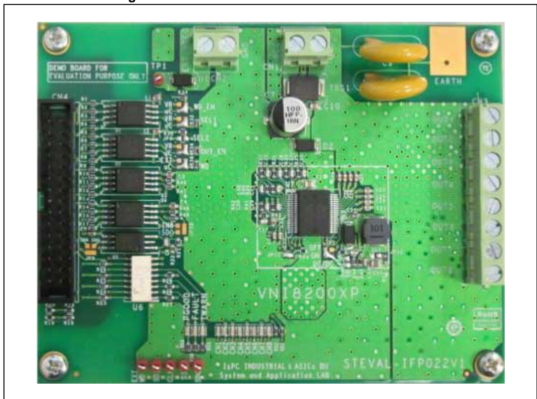
Figure 2. STEVAL-IFP022V1 demonstration board
