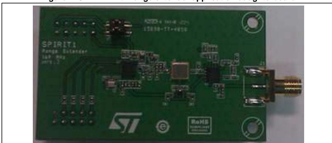
Figure 2. SPIRIT1 application daughterboard plugged into the motherboard
