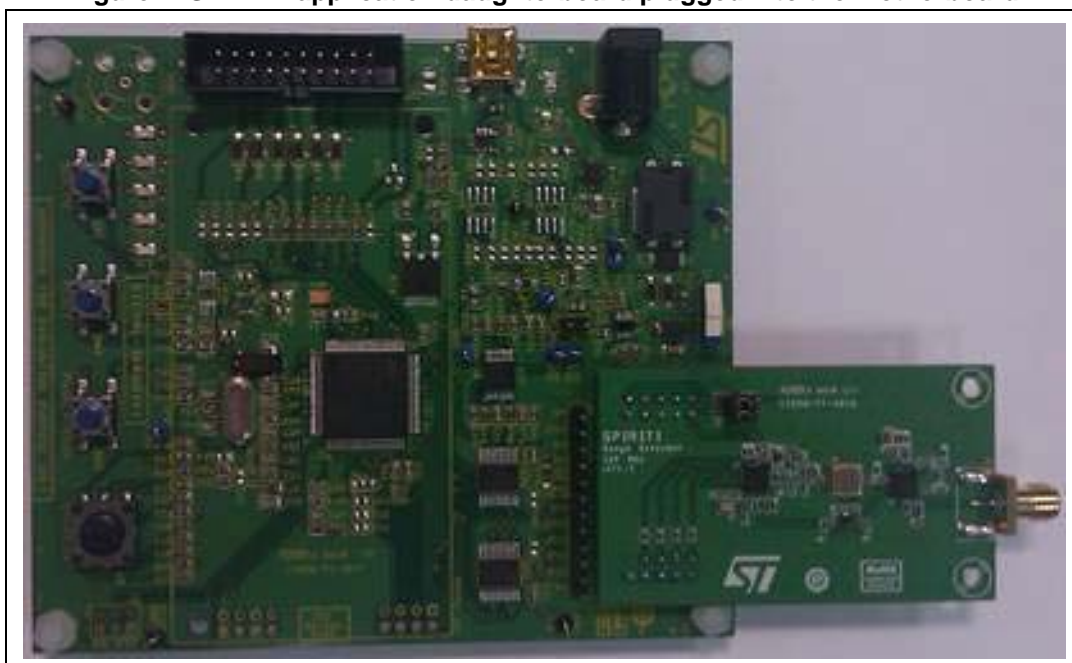
Figure 2. SPIRIT1 application daughterboard plugged into the motherboard
