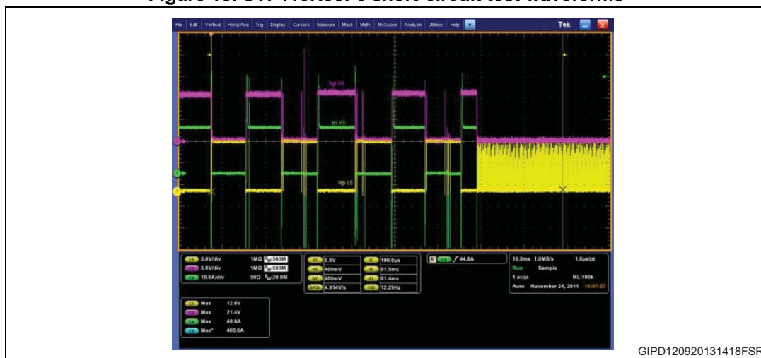
Figure 13. STP110N55F6 short-circuit test waveforms
