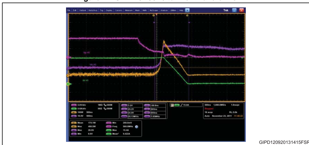
Figure 12. STP110N55F6 turn-off waveforms
