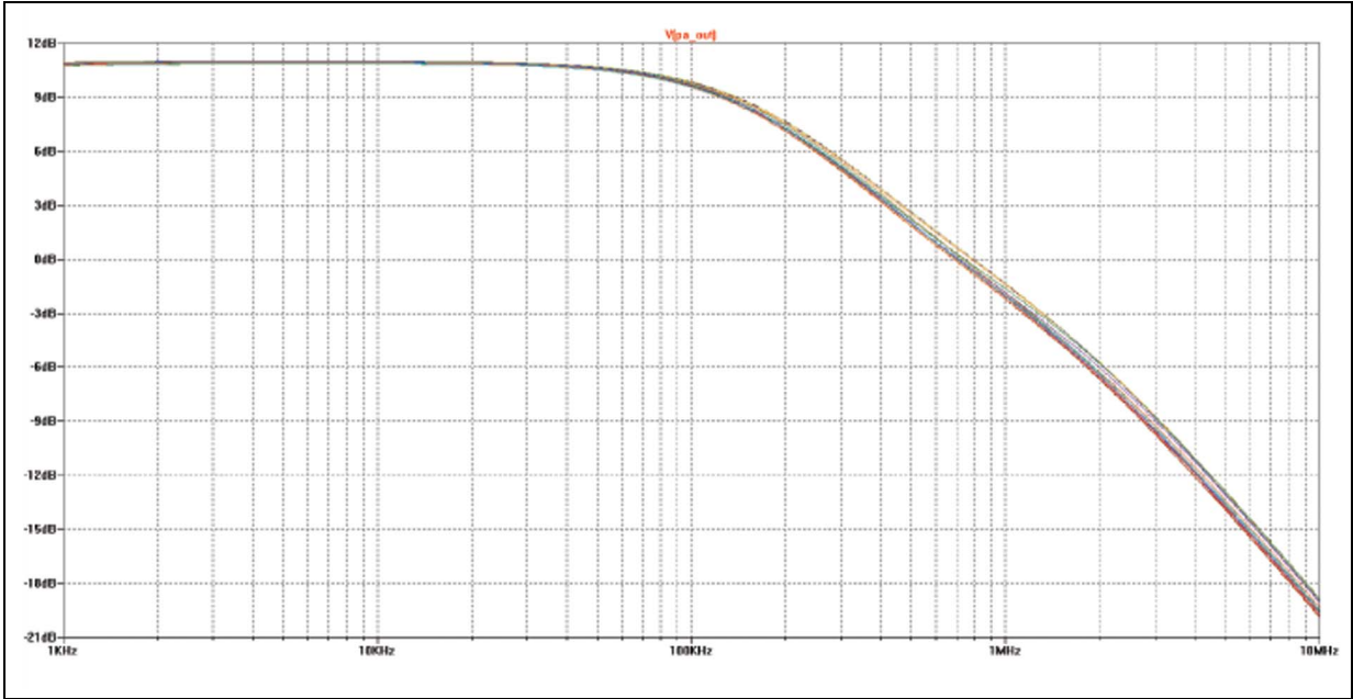
Figure 15. Montecarlo simulation of the line driver frequency response
