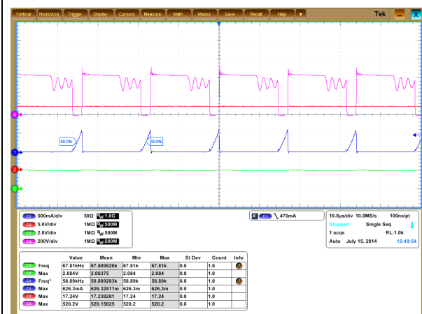
Figure 16. Waveform at 265 V AC
