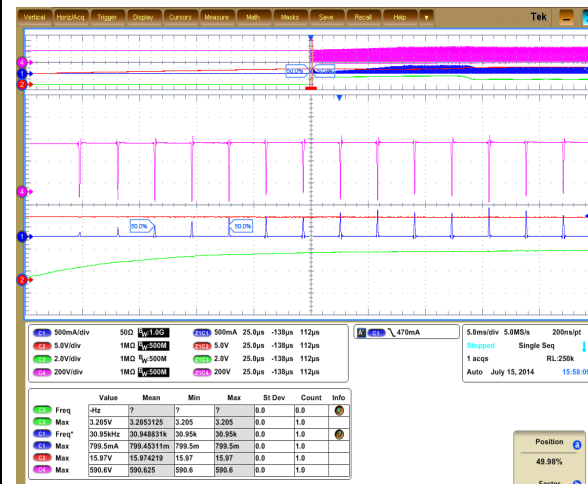
Figure 22. Waveform of start-up at 265 V AC (zoom view 1)
