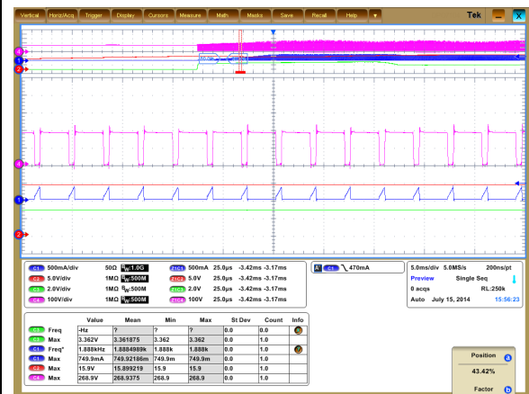
Figure 20. Waveform of start-up at 90 V AC (zoom view 2)
