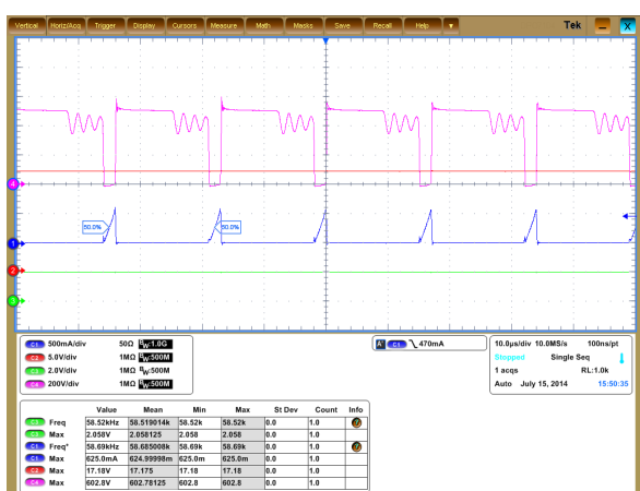
Figure 17. Waveform at 320 V AC
