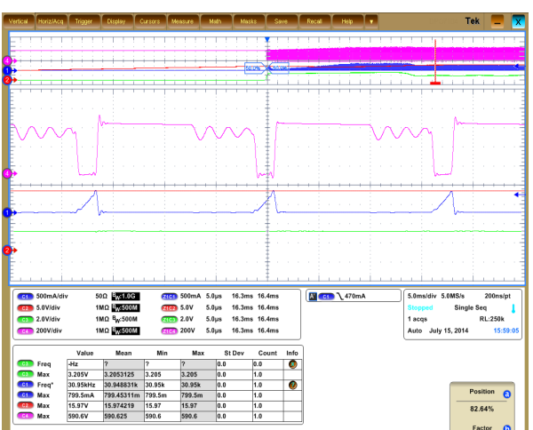
Figure 23. Waveform of start-up at 265 V AC (zoom view 2)
