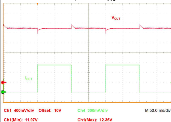
Figure 18. Dynamic step load (0 to 100% output load) at 115 V AC
