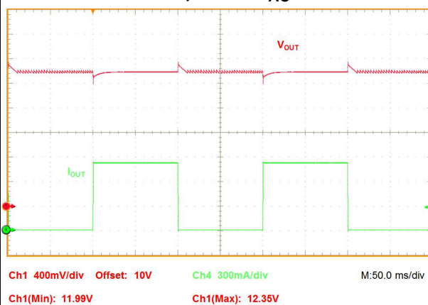
Figure 19. Dynamic step load (0 to 100% output load) at 230 V AC
