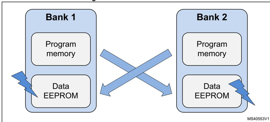
Figure 2 shows the ideal situation in which the code in bank 1 uses data EEPROM from bank 2 and code from bank 2 uses data EEPROM from bank 1 (a similar scenario is registered when program memory to be written is the one of the other bank).
