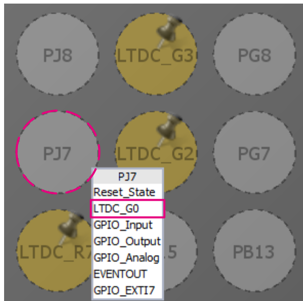
Figure 38. STM32CubeMX: PJ7 pin configuration to LTDC_G0 alternate function
