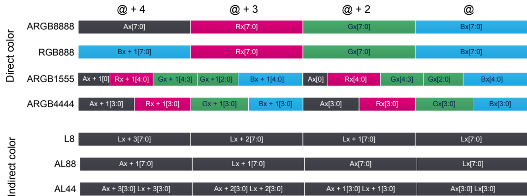
Figure 19. Pixel data mapping versus color format
