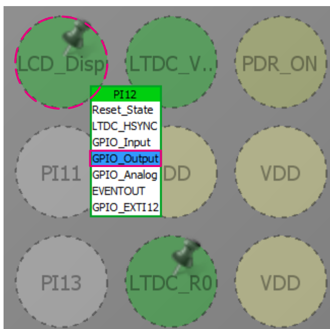
Figure 41. STM32CubeMX: display enable pin (LCD_DISP) configuration
