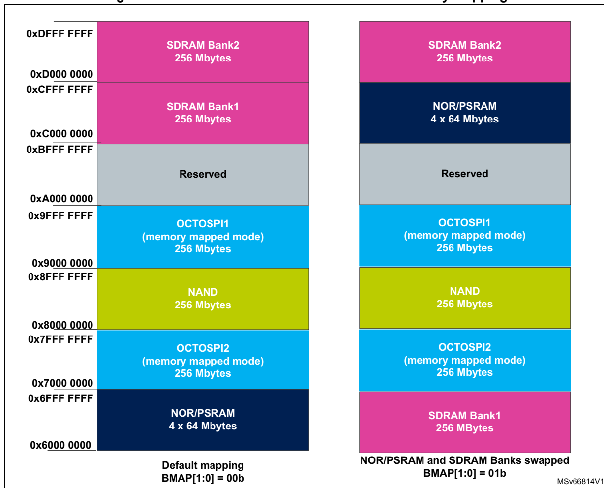
Figure 5. STM32H72x and STM32H73x external memory mapping
