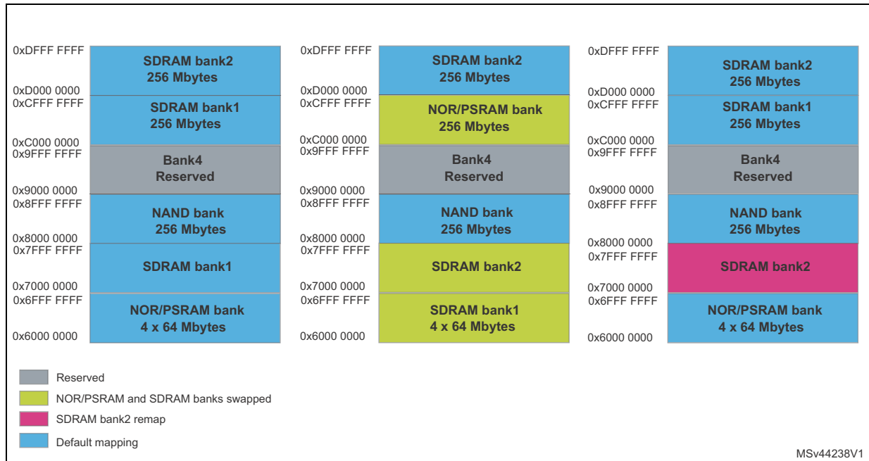
Figure 7. FMC bank address mapping on STM32H7x3 line devices
