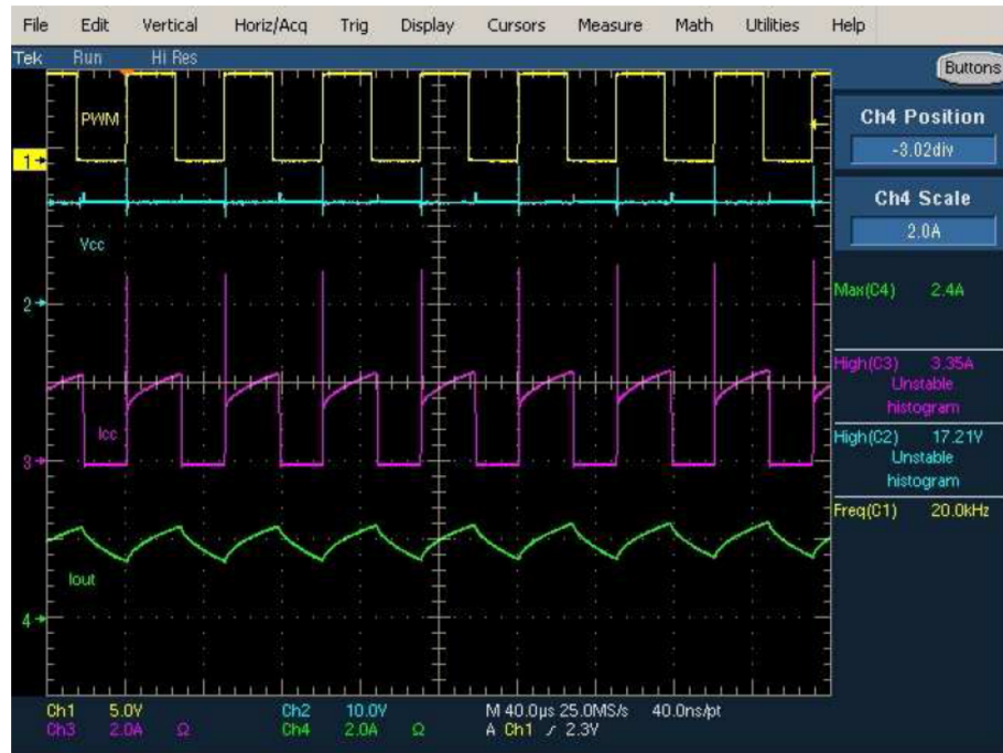
Figure 15. V batt =13.5V, T J =25°C, Duty Cycle 50%, DC MOTOR (CH1=VPWM, CH2=V CC , CH3=I(V CC ), CH4=I motor )
