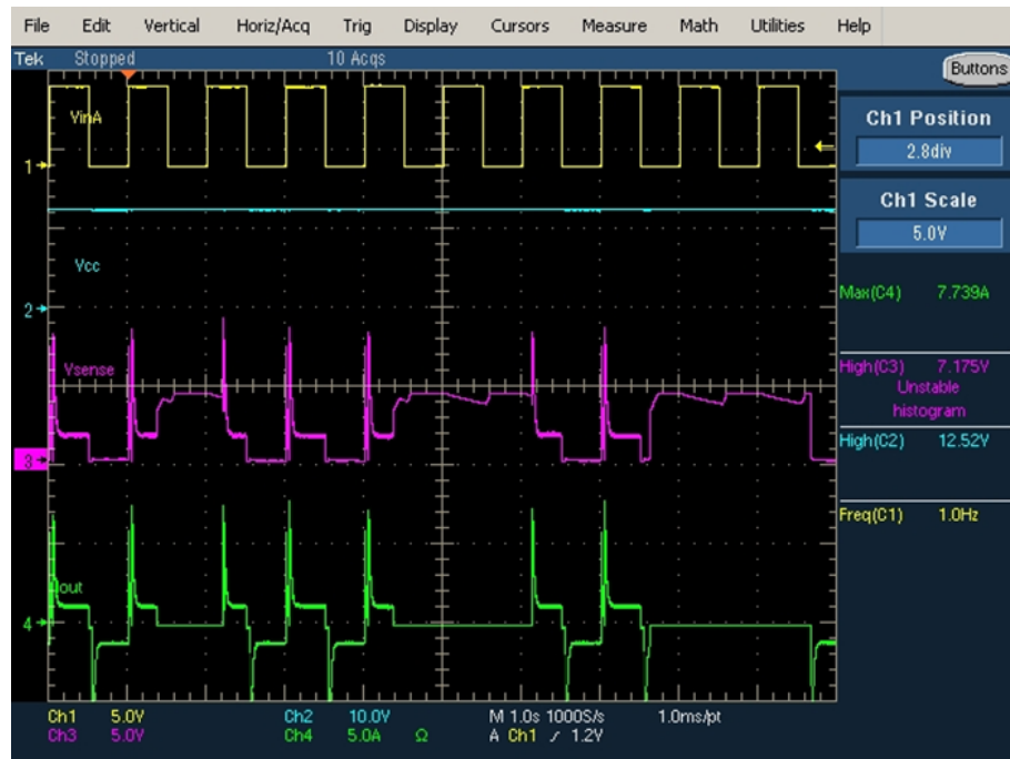
Figure 7. GND loss (INA, Iout, Vbatt, Vsense)
