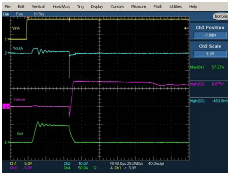
Figure 12. VNH7040AY short across load event (HSA switched on while LSB is already ON)
