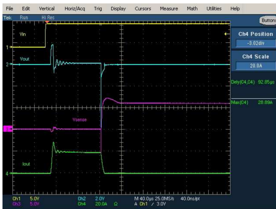
Figure 9. Power Limitation event (VINA, VoutA, Vsense(SEL0=1), Iout=Ihsd)
