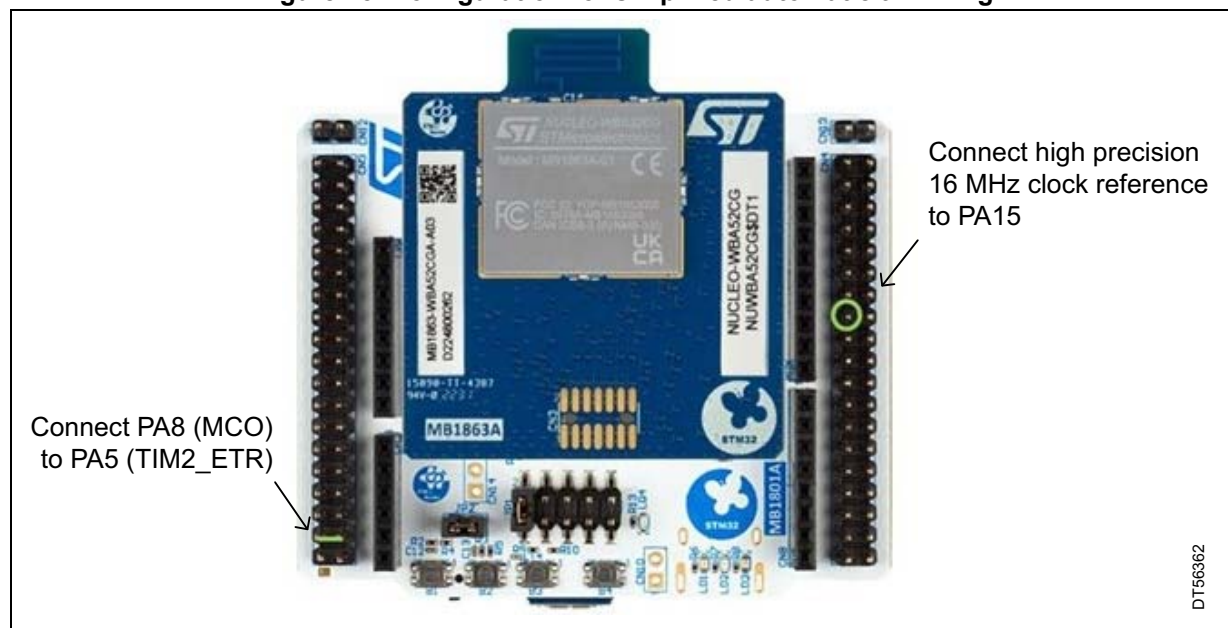
Figure 15. Configuration for simplified automatic trimming
