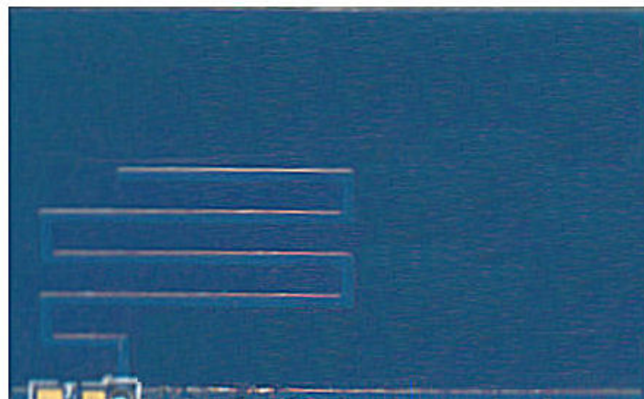
Figure 4. Part of 802.15.4 and BLE PCB with meander-like antenna (scale approximately 4:1)
