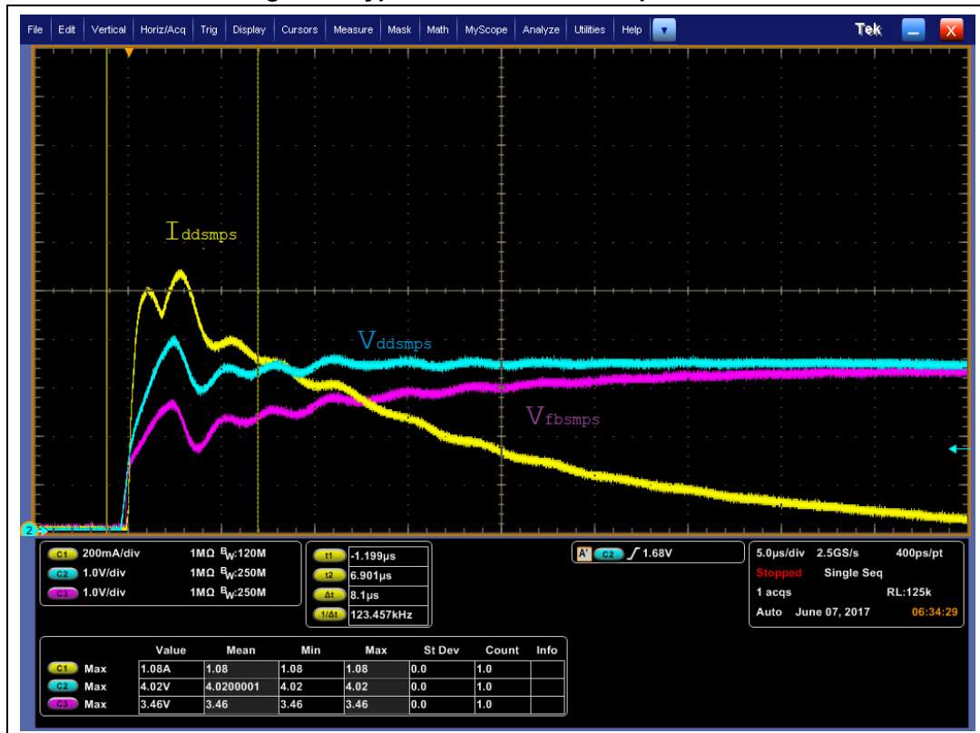
Figure 4. Typical inrush current at power-on
