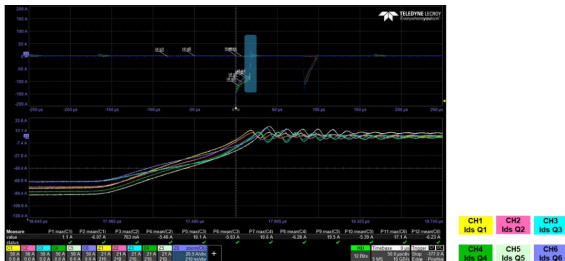
Figure 30. 5 kW inverter active free-wheeling and body drain diode involvement
