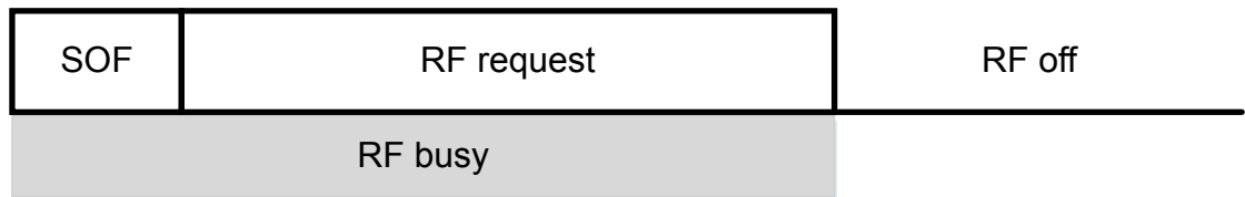
Figure 15. RF busy state for any command when ST25DVxxK exists the RF field
