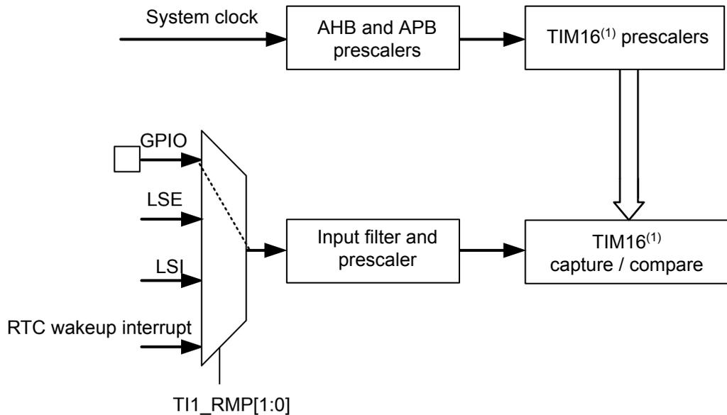
(1) When using an external signal as a reference, another timer can be used instead of TIM16. The firmware provided with this application note uses TIM16
