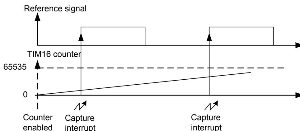
After enabling the timer counter, the timer counter period is captured when the first rising edge of the reference signal occurs and stored in IC1ReadValue1. At the second rising edge, the timer counter is captured again and stored in IC1ReadValue2. The elapsed time between two consecutive rising edges (IC1ReadValue2 - IC1ReadValue1) represents an entire period of the reference signal.
