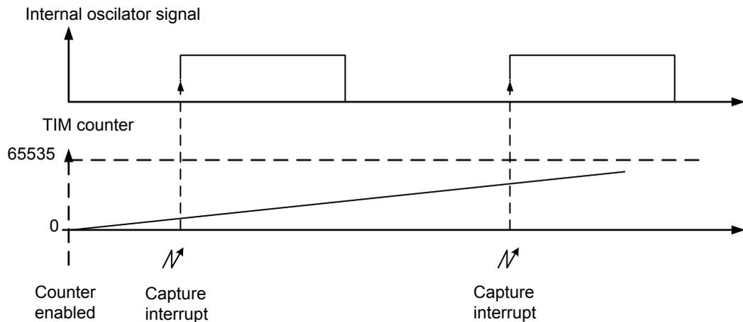
The internal oscillator frequency value is computed as shown in the following formula:
