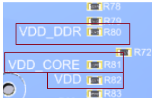
Figure 1. Resistors to be replaced for current measurement
