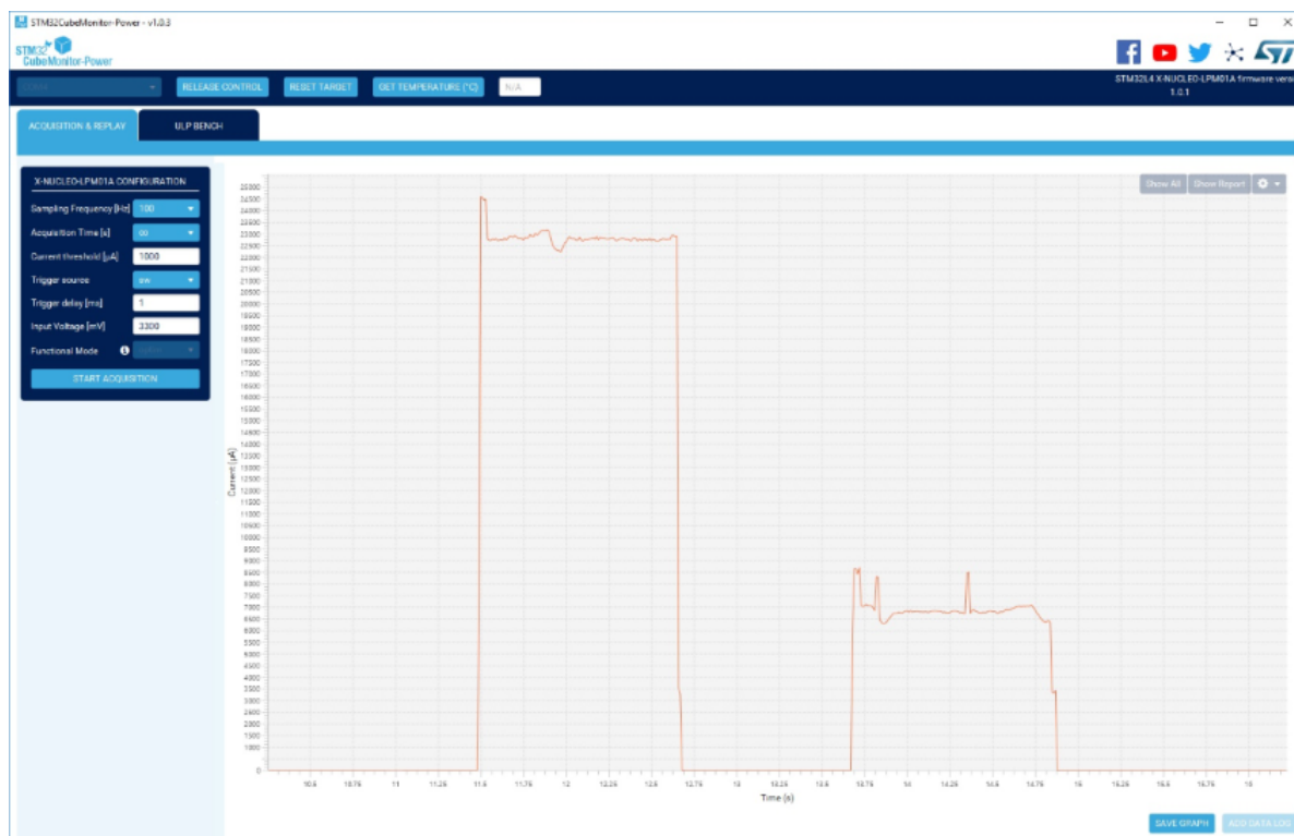
Figure 21. NUCLEO-WL55JC1 current consumption versus time
