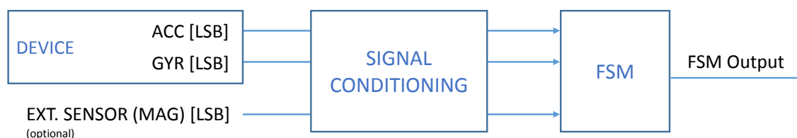
Figure 2. State machine in the LSM6DSO32
