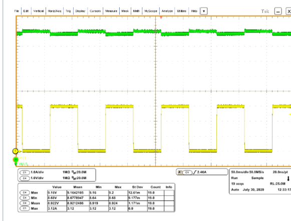
Figure 13. Dynamic load at 9 V/3 A, V_{IN} = 115\text{ V}_{AC}
