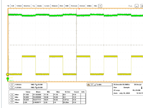
Figure 15. Dynamic load at 11 V/2.45 A, V_{IN} = 115\text{ V}_{AC}
