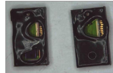
Example of de-soldering at 350°C
