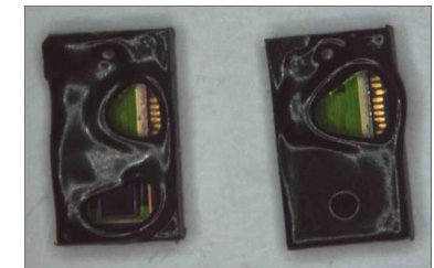
Example of de-soldering at 350°C
