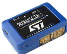
Bluetooth LE enabled wireless IoT node
