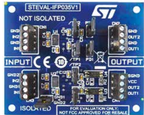
Figure 9 - The STEVAL-IFP035V1 evaluation board for the CLT03-2Q3 series of self-powered current limited termination devices (source ST)
