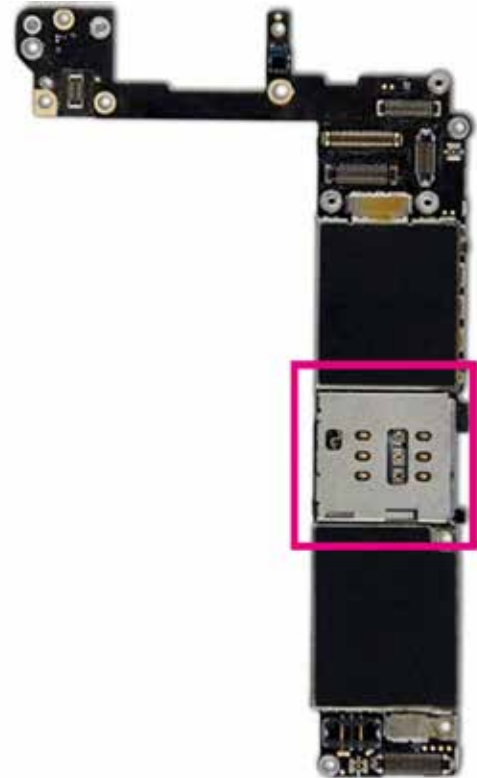
Figure 2. iPhone 6S motherboard with SIM slot
