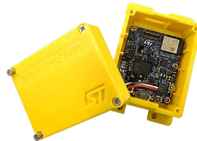
Industrial sensor evaluation kit for condition monitoring based on a 2.4 GHz multiprotocol wireless ultra-low-power STM32WB module (STEWAL-PROTEUS1)
