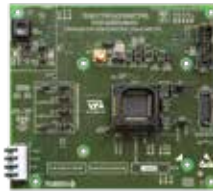
Daughterboard For package adaption & clip-on package
