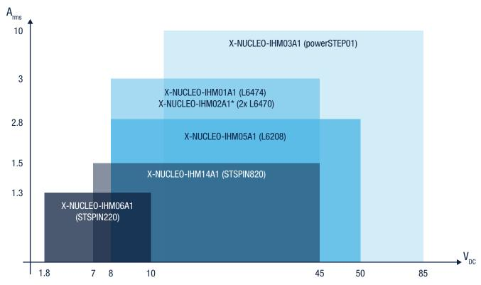
Stepper motor control Nucleo expansion boards grouped by operative range and family. Use this graphical representation to select the best appropriate board based on the operative range of the motor to be used.
