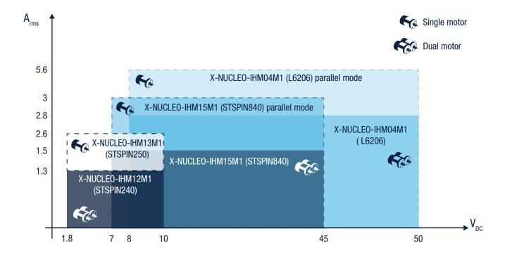
Brushed DC motor control Nucleo expansion boards grouped by operative range and family. Use this graphical representation to select the best appropriate board based on the operative range of the motor to be used.
