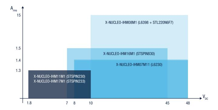
Brushless DC motor control Nucleo expansion boards grouped by operative range and family. Use this graphical representation to select the best appropriate board based on the operative range of the motor to be used.
