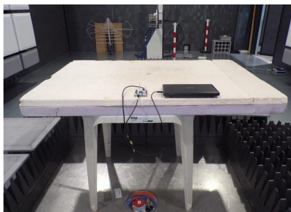
Test setup in full anechoic room (1-2GHz) (semi anechoic room with absorbers on the floor)
