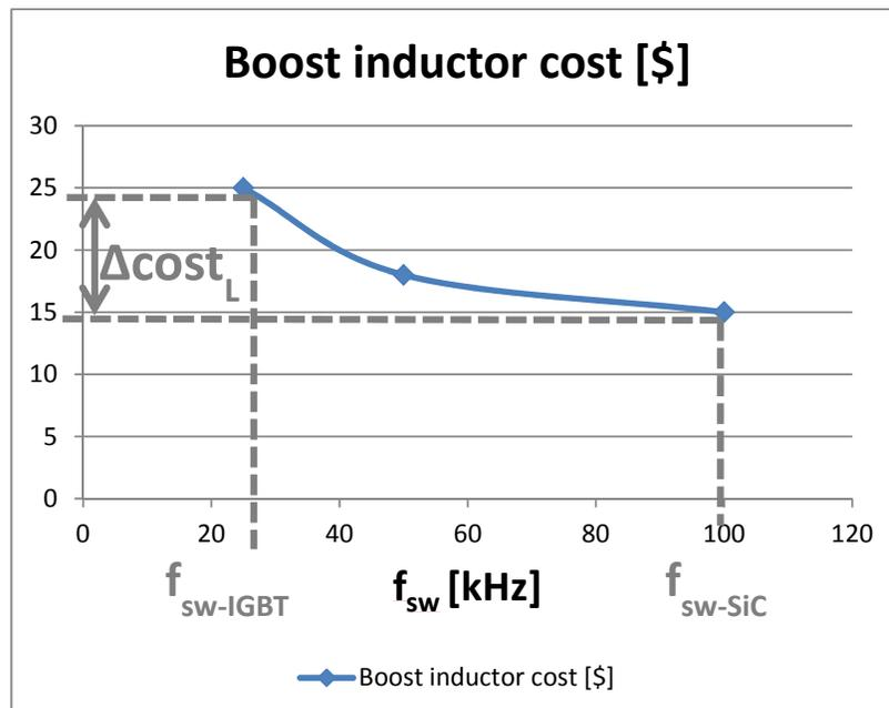
Fig.3. Typical cost of the inductor vs switching frequency
