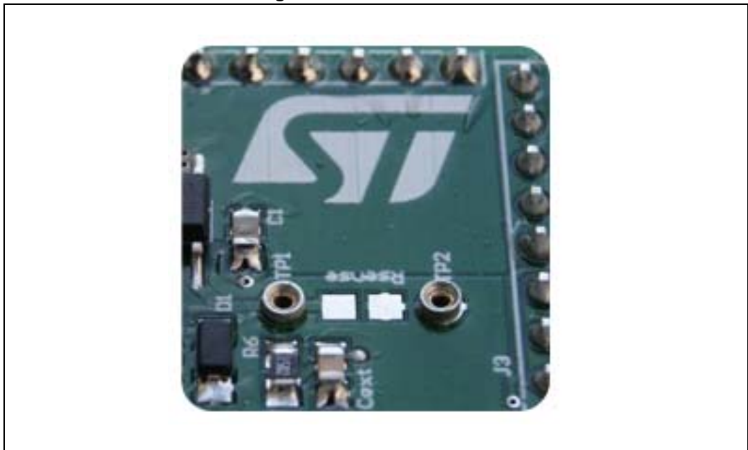
Figure 4. Mounting through-hole sense resistor
