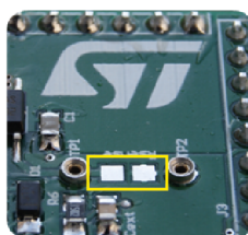
Figure 5. Pads for soldering SMD resistor
