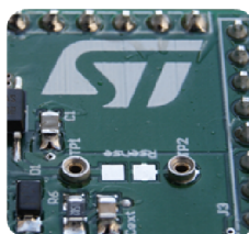
Figure 4. Mounting through-hole sense resistor
