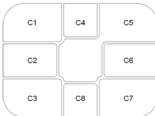
Figure 2. D18 micromodule contact assignment
