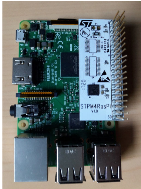
Figure 4. STPM4RasPI embedded in the Raspberry Pi box with touch screen
