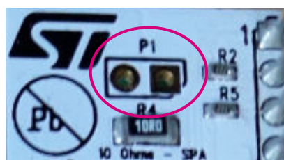
Figure 5. P1 header location
