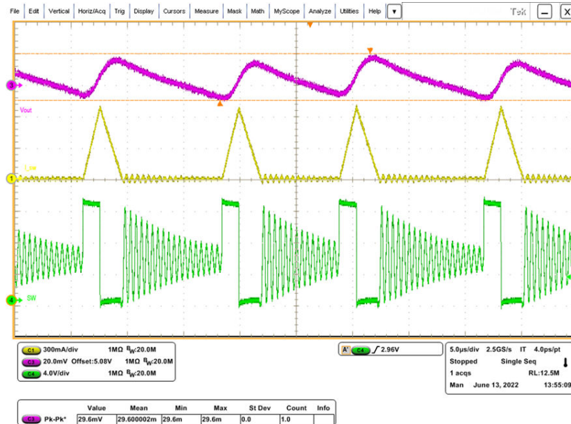
Figure 12. LCM operation over 100 mA load condition (part 3-pulse skipping)
