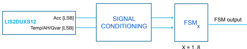
Figure 12. State machine in the LIS2DUXS12
