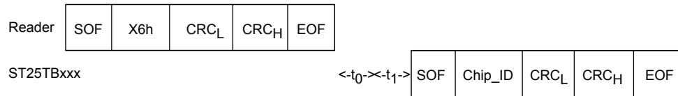
Figure 49. Slot_marker frame exchange between reader and ST25TB512-AC
