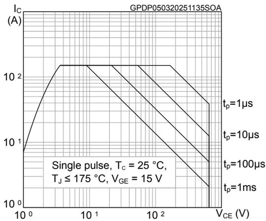
**Figure 10. TO-247 long leads forward bias safe operating area**
