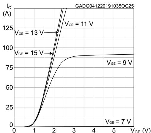
**Figure 6. Typical output characteristics (T\_J = 175 °C)**
