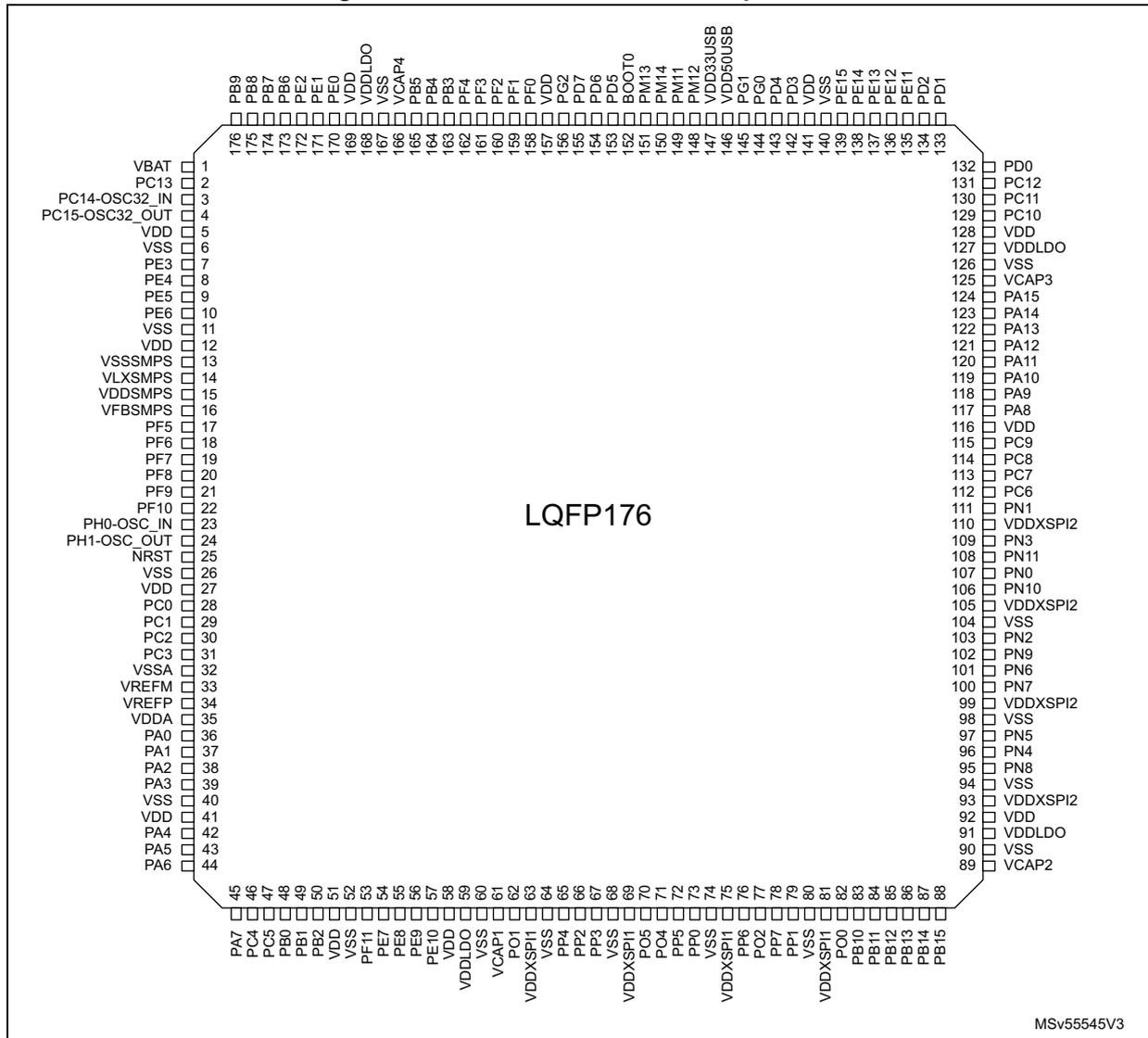
a. The above figure shows the package top view
