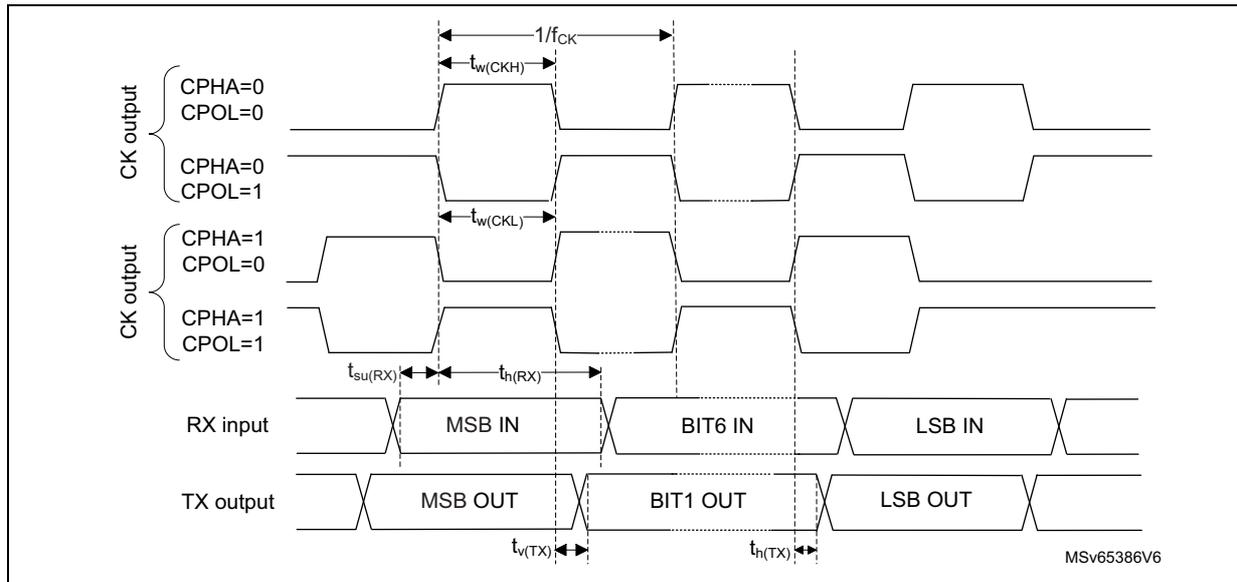
1. Measurement points are done at  $0.5V_{DD}$  and with external  $C_L = 30\text{ pF}$ .
