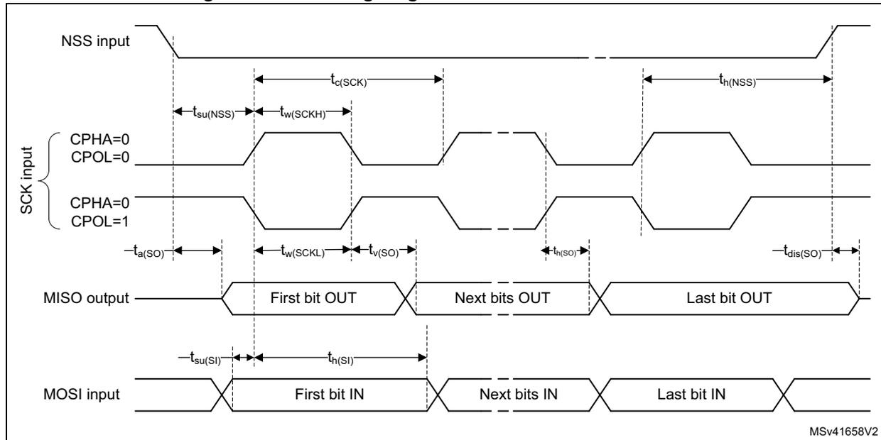
Figure 64. SPI timing diagram - slave mode and CPHA = 1
