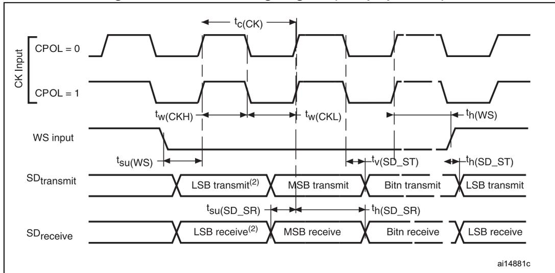
1. LSB transmit/receive of the previously transmitted byte. No LSB transmit/receive is sent before the first byte.
