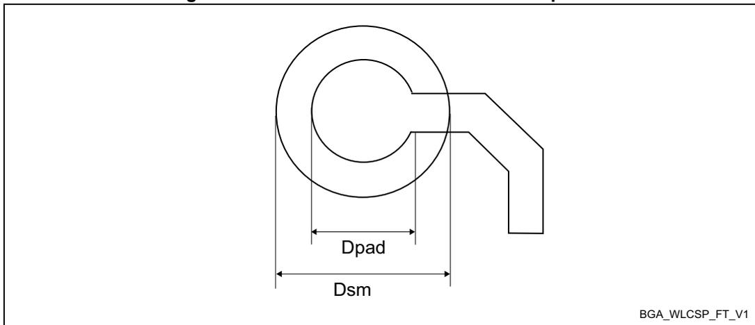
**Table 147. UFBGA144 - Recommended PCB design rules (0.80 mm pitch BGA)**
