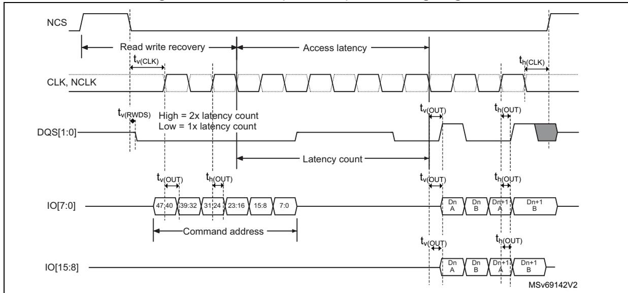
Figure 53. XSPI DTR (with DQS) read timing diagram
