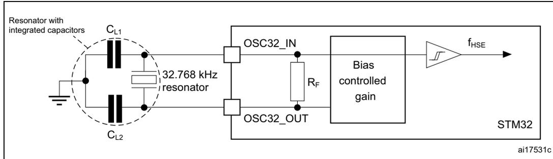
1. An external resistor is not required between  $OSC32\_IN$  and  $OSC32\_OUT$  and it is forbidden to add one.
