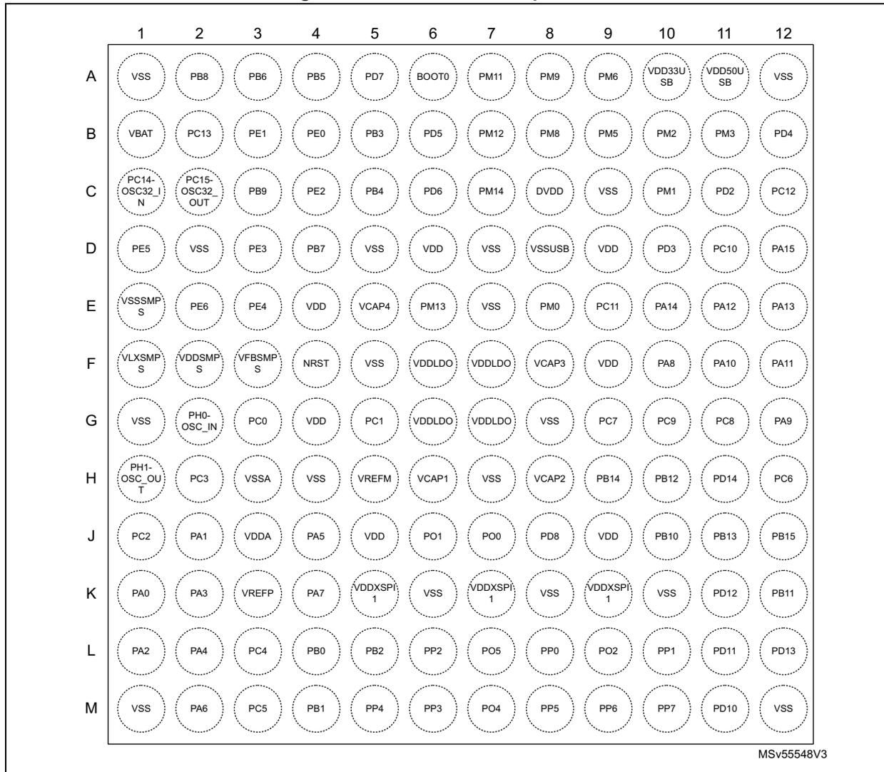
a. The above figure shows the package top view.
