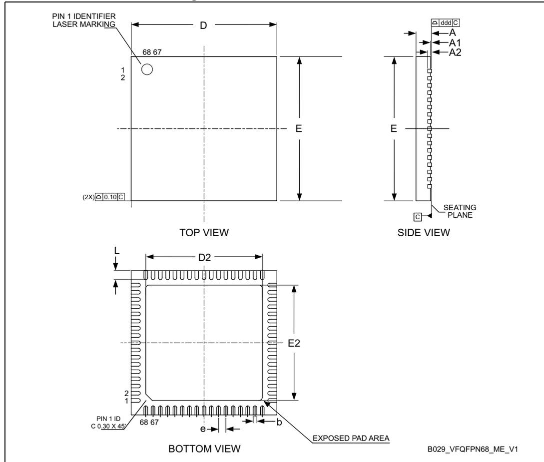
1. VFQFPN stands for Thermally Enhanced Very thin Fine pitch Quad Flat Packages No lead. Sawed version. Very thin profile:  $0.80 < A \leq 1.00\text{mm}$ .
