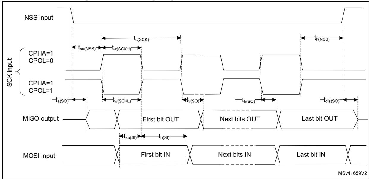
Figure 65. SPI timing diagram - master mode
