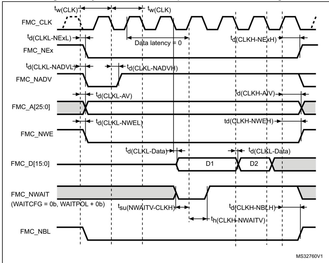
Table 91. Synchronous multiplexed NOR/PSRAM read timings<sup>(1)</sup>
