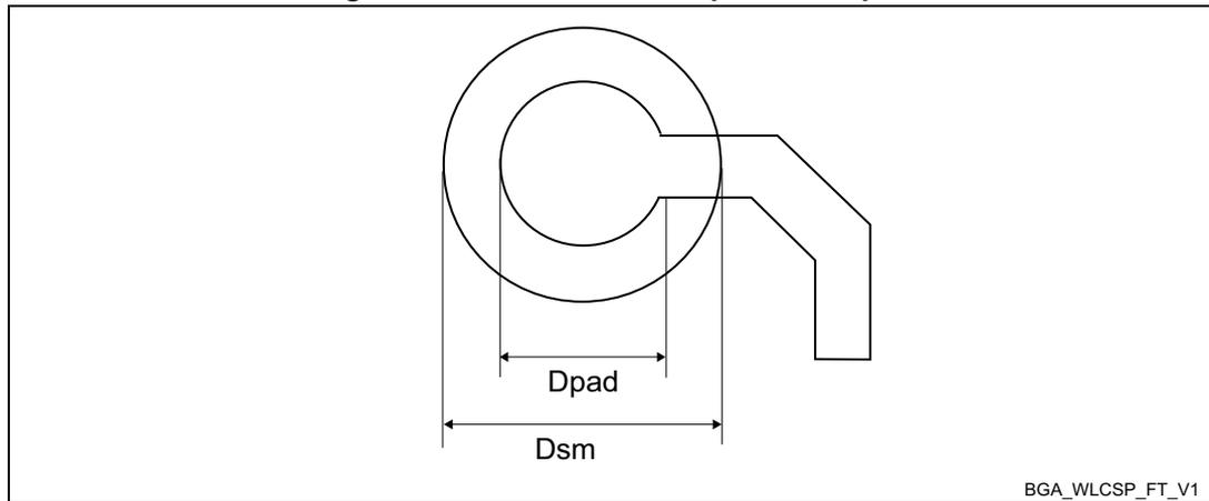
**Table 156. TFBGA225 - Recommended PCB design rules (0.8 mm pitch BGA)**
