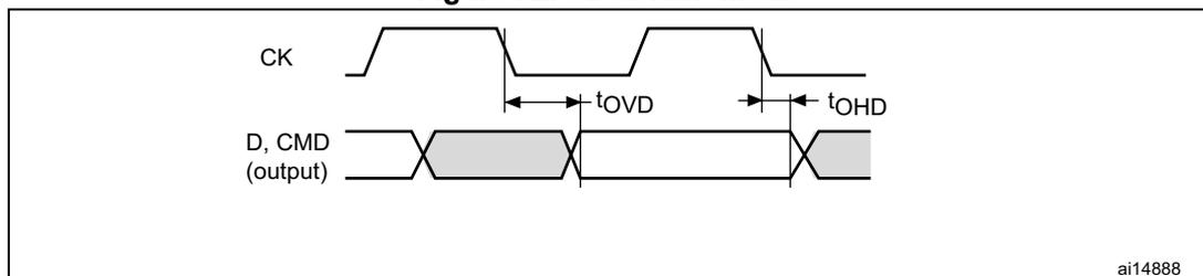
Figure 73. SDMMC DDR mode
