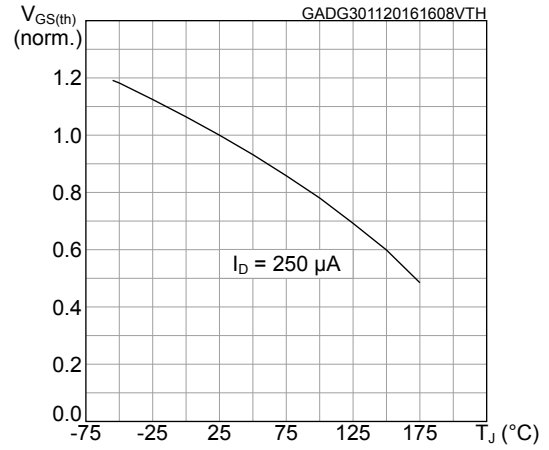
Figure 8. Normalized gate threshold voltage vs temperature
